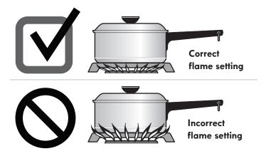
For most cooking: start on the highest setting and then turn to a lower setting to complete the process. Use the recommendations below as a guide for determining proper flame size for various types of cooking (Fig. 2)
